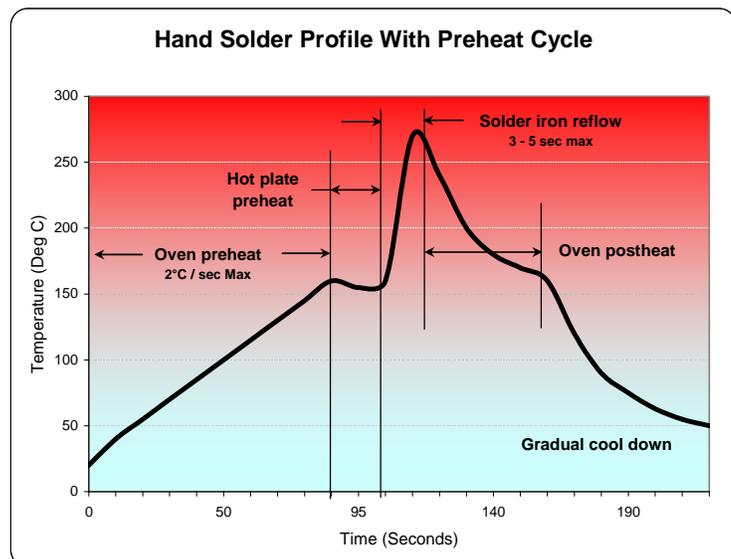
Figure 2 – Soldering Profile / Recommendations
