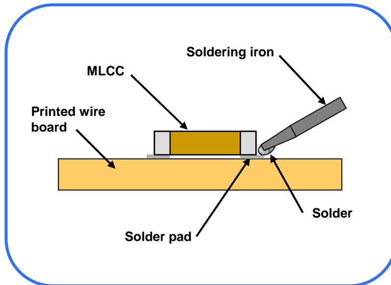
Figure 4 – Hand Soldering Technique
