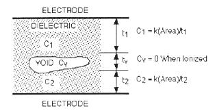
Figure 2. Equivalent Capacitors at Ionized Void
