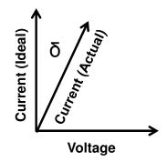
Figure III: Loss Tangent for Practical Capacitor
